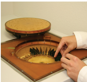
Placing the coupons inside a HATS tester
